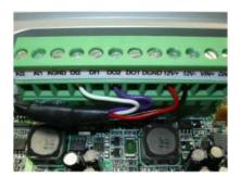
NOTE: The DI2 input debounce link must be removed for the SDI-12 function to work correctly. See the section above (Section 13.2) shows the link positions on the V1.1 PCB.
